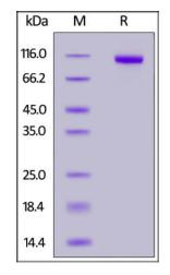
Rabbit PTK7, His Tag on SDS-PAGE under reducing (R) condition. The gel was stained with Coomassie Blue. The purity of the protein is greater than 95%.
