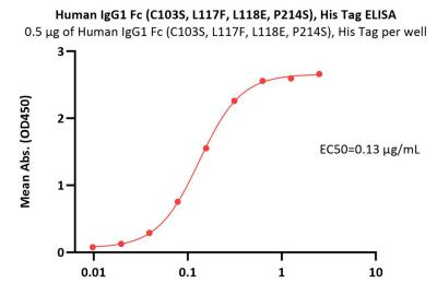
Immobilized Human IgG1 Fc (C103S, L117F, L118E, P214S), His Tag (Cat. No. IG1-H52H9) at 5  $\mu$ g/mL (100  $\mu$ L/well) can bind Biotinylated Human CD64, His,Avitag (Cat. No. FCA-H82E8) with a linear range of 0.01-0.625  $\mu$ g/mL (QC tested).
