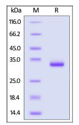
Human IgG1 Fc (C103S, L117F, L118E, P214S), His Tag on SDS-PAGE under reducing (R) condition. The gel was stained with Coomassie Blue. The purity of the protein is greater than 95%.
