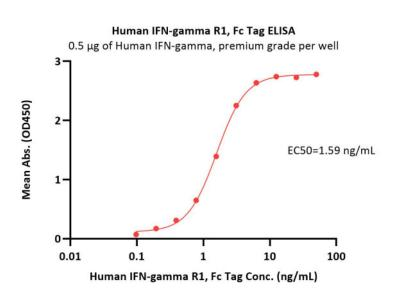
Immobilized Human IFN-gamma, premium grade (Cat. No. IFG-H4211) at 5  $\mu$ g/mL (100  $\mu$ L/well) can bind Human IFN-gamma R1, Fc Tag (Cat. No. IF1-H5254) with a linear range of 0.1-6 ng/mL (QC tested).
