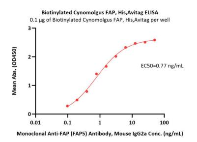
Immobilized Biotinylated Cynomolgus FAP, His,Avitag (Cat. No. FAP-C82Q5) at 1  $\mu$ g/mL (100  $\mu$ L/well) on streptavidin (Cat. No. STN-N5116) precoated (0.5  $\mu$ g/well) plate can bind Monoclonal Anti-FAP (FAP5) Antibody, Mouse IgG2a with a linear range of 0.1-2  $\mu$ g/mL (QC tested).
