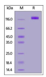
Human EGF R, Llama IgG2b Fc Tag on SDS-PAGE under reducing (R) condition. The gel was stained with Coomassie Blue. The purity of the protein is greater than 95%.
