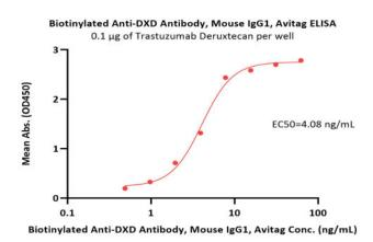
Immobilized Trastuzumab Deruxtecan at 1 µg/mL (100 µL/well) can bind Biotinylated Anti-DXD Antibody, Mouse IgG1, Avitag (Cat. No. DXD-BVM807) with a linear range of 0.5-8 ng/mL (Routinely tested).
