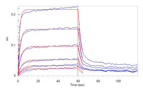
Loaded Human BAFF Protein, Fc Tag (Cat. No. BAF-H5261) on Protein A Biosensor, can bind Biotinylated Human BCMA, His,Avitag (Cat. No. BCA-H82E4) with an affinity constant of 0.69  $\mu$ M as determined in BLI assay (ForteBio Octet Red96e) (Routinely tested).
